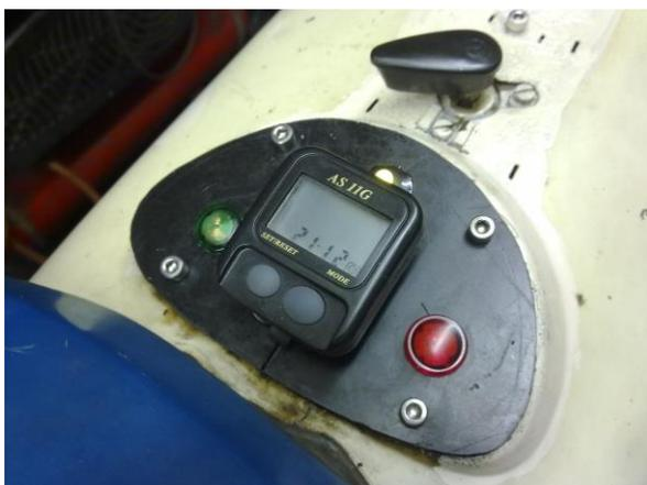
The green warning light is for Neutral and the Red light covers both the charge light and the brake warning light should the fluid level drop. As far as I can see there is no reason not to combine the functions. Obviously if the light does come on whilst running, I will not know if I have a charging problem or a brake fluid problem. However, in either case I need to stop and investigate. The yellow LED just in front of the speedo is the main beam warning light. At
