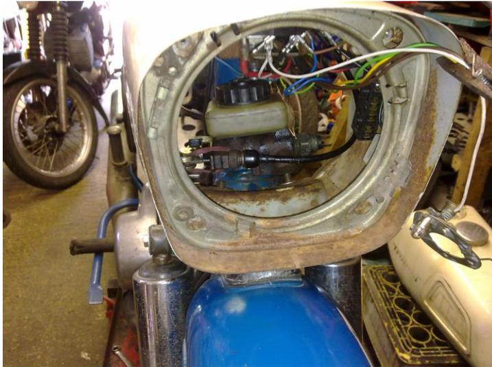
At the handlebar end is just the normal front brake lever and cable which I have adapted from the original BMW cable. No obvious clues from the handlebars about the disk brake. I have ordered a set of Goodridge connectors and pipe which will be here tomorrow. If I get the cable runs correct, it should be possible to remove and replace without needing to disconnect any of the hydraulic connections. I will need to make up a rubber mounted mounting for the
