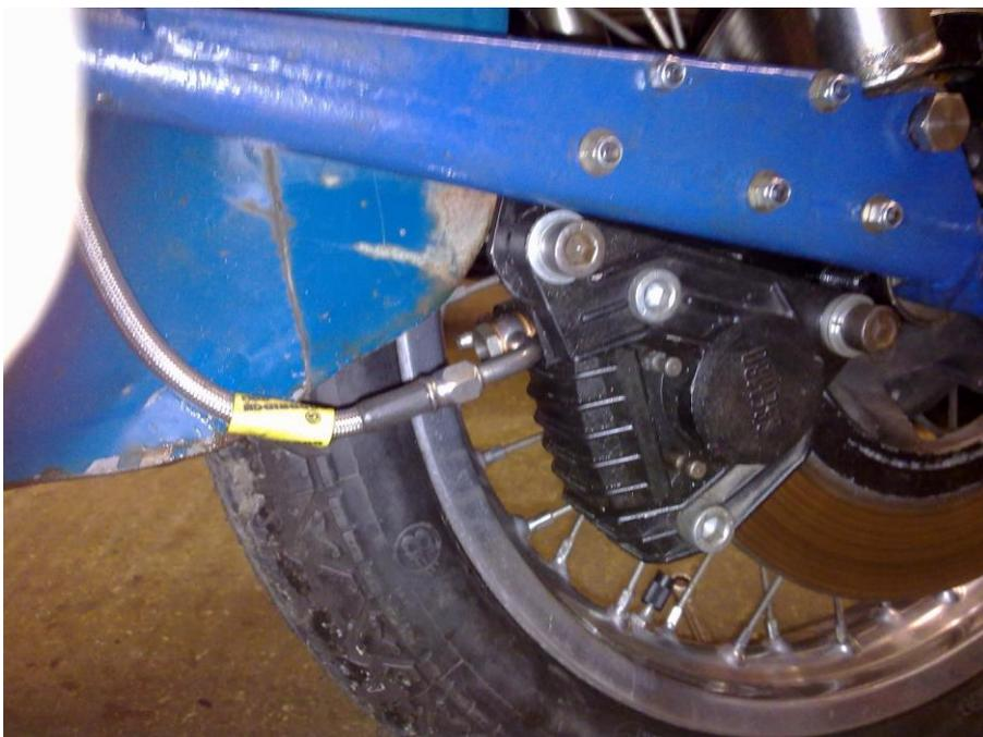
made up a bracket to rubber mount the master cylinder. As usual, I had trouble getting the hydraulics bled properly but in the end it came together. Pushing it round the garage, the brake seemed to work well so I decided to give it a test ride round the garden. First hard application and ping went the new nipple I had
