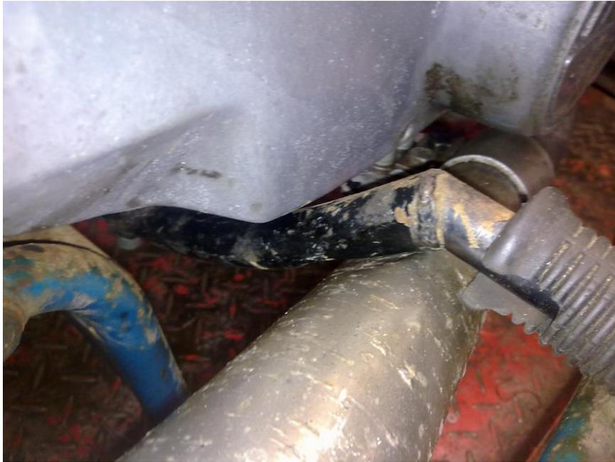
TS250 exhaust pipe and offered these up but found that the silencer fouled the footrest. Strange really as the one I had removed seemed to fit perfectly well. (looking at an early picture later I realise that there was no footrest fitted when I bought the bike). Anyway after making up a spacer bracket and putting a small dint in the silencer, I did get it to fit acceptably.
