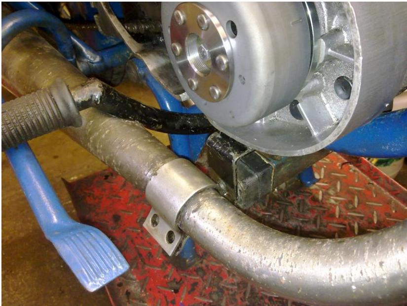
TS250 motor has also been fitted over the past couple of days, This one has been used in an ETS250 frame in the past which uses the same type of engine mounts as the ES250. This engine has an extra lug grafted on the near side crankcase to connect up to the bottom engine plate. Cannot complete the engine installation until the second rubber mount and the chain guides arrive so whilst waiting I decided to fit the
