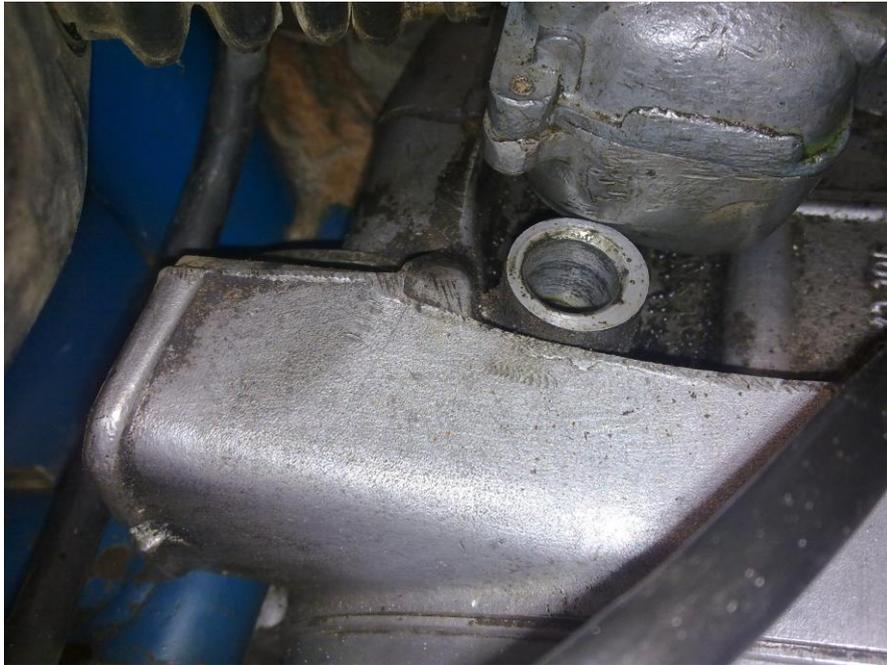
manifold. This also meant fitting an ES250 carb. These are 28mm instead of the 30mm used on the TS250, but more importantly have a smaller diameter spigot to match the ES250 manifold. This is where I hit a rather more difficult snag. The gearbox filler hole on the TS250 engine fouls the carb as the neck is on the opposite side to the ES250 crankcases.
