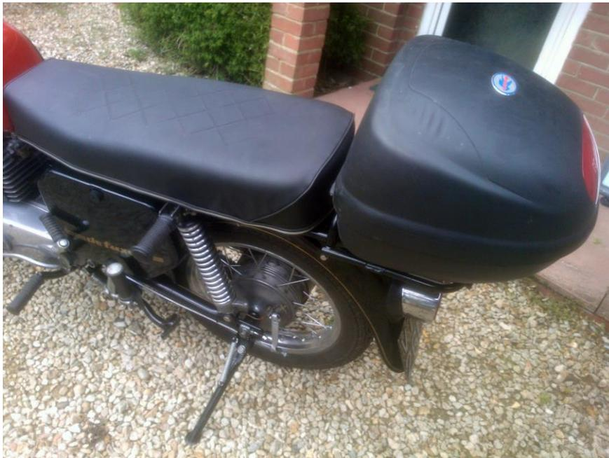
bag of some sort is essential. The top box was borrowed from my TS150 which has a much larger carrier than the soft bag fits much better so a good swap. Though looking at the picture now the top box does look bigger than I had realised. The other change was to fit a passenger footrest assembly onto the top nearside shock mounting. This gives a handle to pull the bike onto the stand. Previously I was using the
