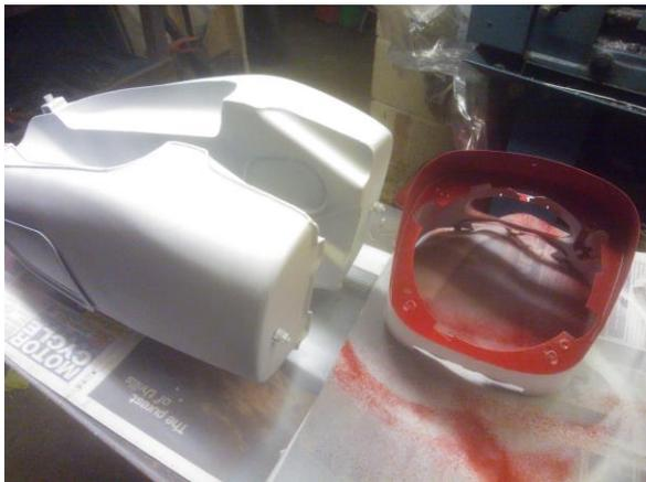
I dug out my HVLP spray gun and managed to get a couple of coats of primer on the headlamp and one coat on the bottom of the tank before it got too cold for serious spraying. I also tried a quick burst with the spray can inside the headlamp
