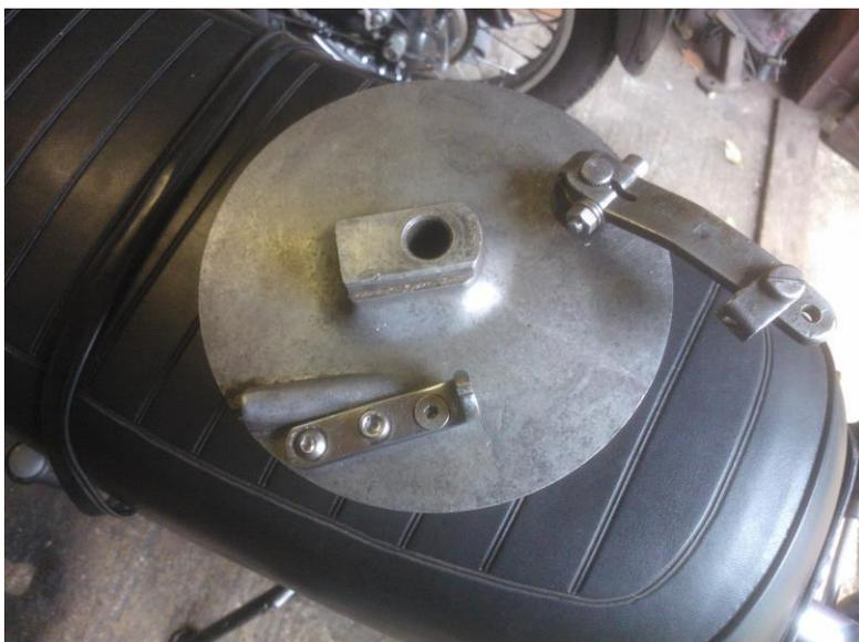
well, I must admit that aesthetically it looks wrong. I do have the original wheel and brake drum so I will clean both up so that I have an option. I have modified the brake plate to use an external brake arm which gives greater leverage. This involves drilling the pivot hole for the original brake cam right through, then using a rear brake cam which is much longer; in fact too long really. Mine has been
