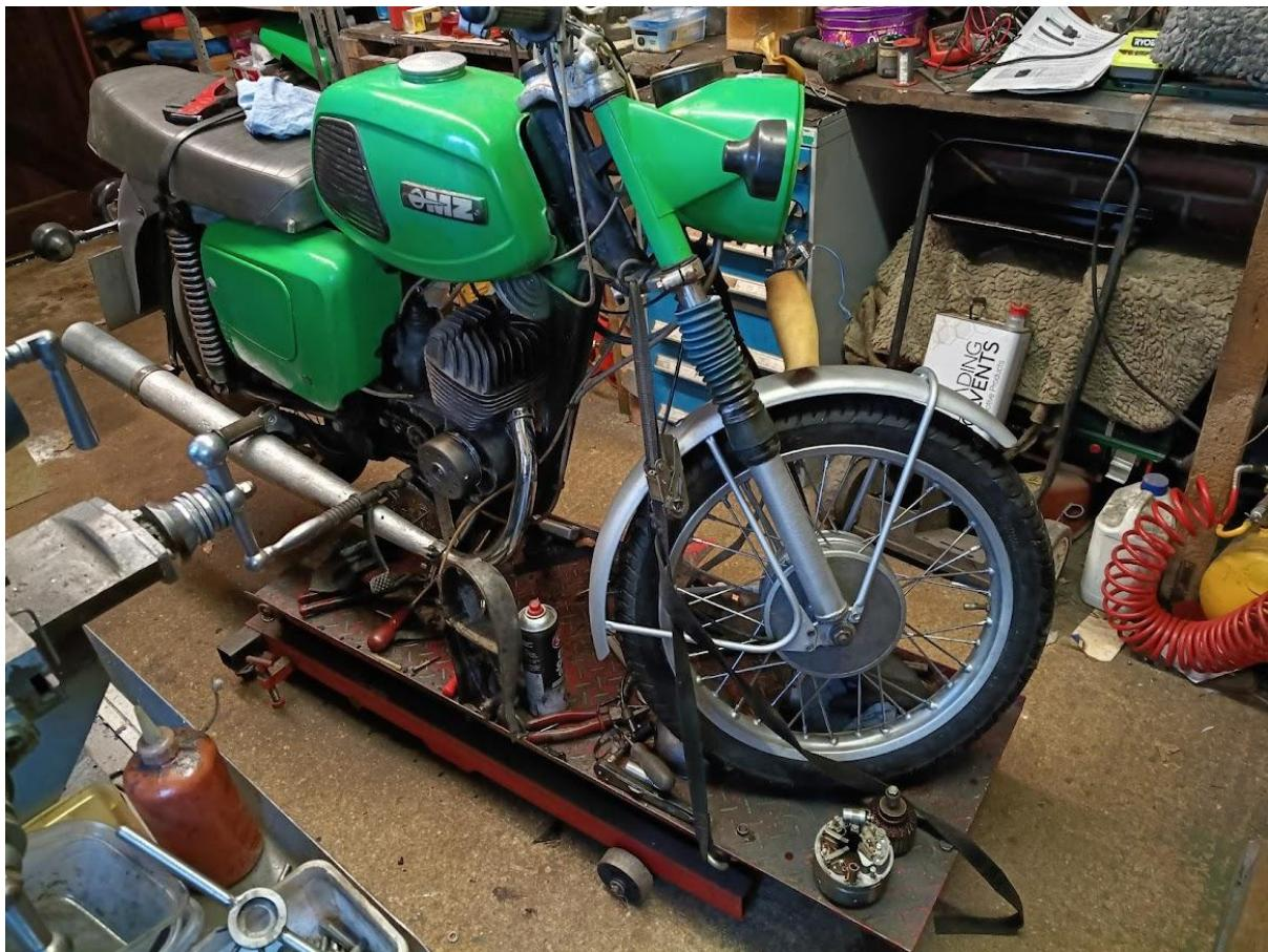
The next task was to fit a rear carrier, the one I removed from the yellow TS150; not too difficult. The final task was to fit a 16t gearbox sprocket. This threw up a problem. What I thought was a 16t TS150 sprocket was too wide, probably 428 chain rather than 420 and was less dished. The chain also looked tired. Time to find out what a new chain and sprocket will cost and decide whether to replace or just put it all back for now.
