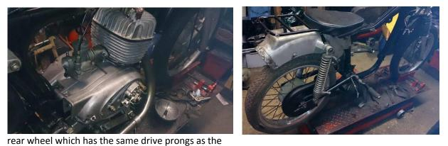
TS150. However, I could not get the wheel into the fork and in any event, it has a 160mm brake drum whereas the TS150 uses a 150mm drum so the brake plate does not fit. For the moment I have dropped this idea but if I can source an ETZ125/150 wheel I may try again as it would help to lower the gearing
