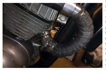
show my shoddy workmanship to Mick the welder. In the post on Thursday I received the exhaust wrap which I ordered earlier in the week so I have now wrapped the pipe and the results can be seen below. Not only does it hide by dodgy welding, but it will stop the rust showing through. If the bike otherwise proves a success, I hope to get a pipe properly made up by Armours or some other specialist using my effort as a template. I have also put a temporary shield on the
