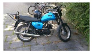
wheels over so that I retained the one with s/s spokes. Nothing wrong with the old Supa5 wheel but it was rebuilt about 9 years ago with chrome spokes and eventually they will start to rust again. By the time they do my grandson will either have moved on to bigger bikes or more likely four wheels. While the Supa5 wheel was out I fitted a newly painted front mudguard as well.
