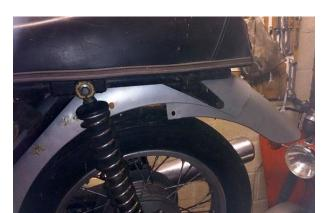
have some leather straps somewhere which I plan to use – just like the ISDT bike. On reflection, I actually prefer this tank arrangent over the stock item. A TS250 rear mudguard was something else which I did not have in stock but an old ETZ250 guard fitted the wrong way round went on ok with a tail piece from a TS150. Not overly satisfied with that arrangement but it will do for now.
