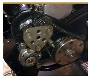
Back home the major task was to fix the Velo starter motor and in this I was quite successful in the end. In theory it was a simple matter of making up a triangular plate and a couple of spacers.
