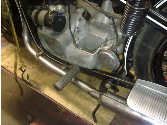
limited by the bell housing, but certainly enough (or so I thought) for operational use. The exhaust system was next and gave me a few headaches. The pipe seems not to be quite the right bend and does not follow the shape of the frame. In part this is due to it fouling the engine mounting bolt so I need to think of a way to slim this down. The silencer is a Chinese pattern item and a very tight fit on the pipe. In fact I had to cut a slot on the inside to get it on at all.
