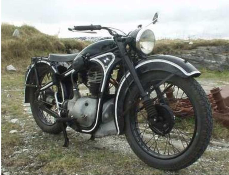
which is commonly called the R35/0. Probably the most significant differences were the front forks which were undamped on the earlier models, the wheel rims which have a very unusual shape and the pressed steel rather than cast front brake plate. These early post war models are referred to as the R35/1 (those mainly built from stockpiled parts) or R35/2. Such models were fitted with the
