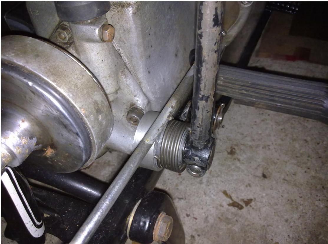
I also removed and had powder coated the footrests and rear brake lever as these were rusty and spoiled the look of the bike. These bits came back a couple of days ago and have now been fitted. Spurred on by this success I finally plucked up courage to take the bike out for a ride today. Apart from a binding back brake caused by forgetting to adjust it after fitting the footrest and brake lever, the bike ran well and we did about 15 steady miles mostly at 30-35 with an occasional burst up to 40.
