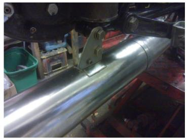
new parts. I was determined this time to use the complete new system but each time I offered it up the result was disappointing. The silencers are identical but the pipes do have a slightly differing bend but whichever side I put them on they did not look right. Eventually I got it all to line up with the mounting holes in the frame but when I looked from the rear the offside silencer was sitting
