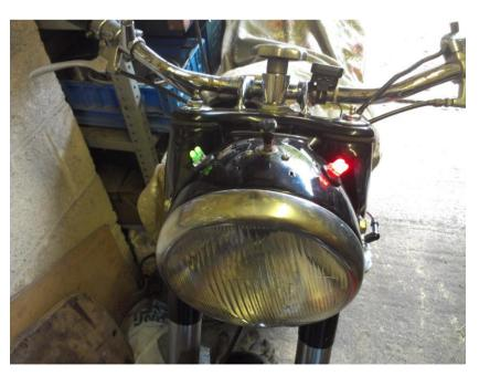
assembly were slim enough to pass trough the cup holder and a couple of rubber grommets neatly sealed the hole. Not a wonderful job but much neater than my first attempt. The only snag was that in my haste to fit them, I forgot to seal the assembly with araldite to make it waterproof so I will have to partially dismantle them some time. It's not urgent as
