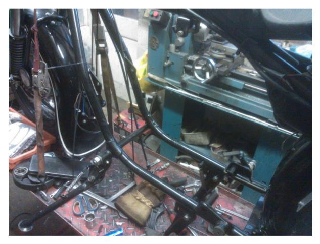
To my surprise the engine gearbox assembly was relatively easy to remove from the frame as a unit by myself though getting it back in with damaging the paintwork is definitely a two person job. Getting the gearbox of was just a question of undoing four nuts and it pulled clear. At some stage it will need some serious investigation as most of the oil I put in when I
