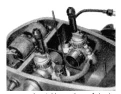
the other was about 4 turns out. Both are now et to 2 ½ turns out also per the manual. The throttle slide arrangement is quite unique and not just because of the flat slides. The slide is actually operated by a rod which terminates in a special housing which also locates the throttle cable. This complex arrangement is needed to allow the top cover to be removed and replaced easily. There are also buttons built into the top cover to
