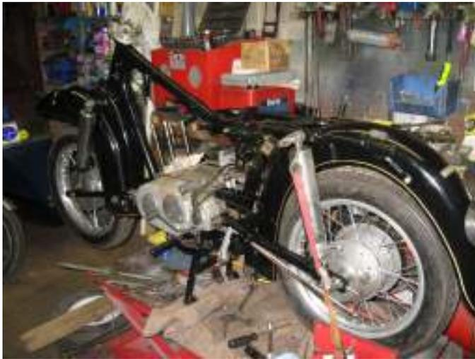
bit worried about clearance for the exhaust system. Fitting the rear mudguard and rear wheel was simple enough, though I found that I had overlooked painting the rear torque arm so this will have to be done later. With the wheel in place I was also able to fit the rear brake pedal and line up the rest of the brake connections. Final job of the day was to fit the airbox, which also provides the mounting for the coil, regulator and fuse box. So
