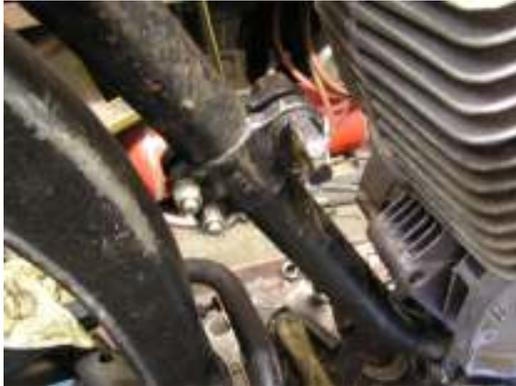
straight struts were relatively simple. The front one mated to a 40mm clamp on the front down tube. I was fortunate to have one of these already in the garage.
