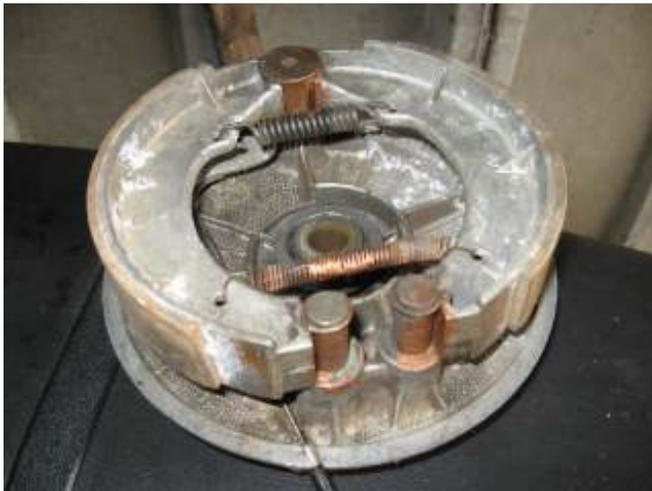
fitting the brake back-plate, I noticed that someone had modified the brake shoes. They normally pivot on pins at the back but these had been filed flat so that they can slide on the pins. In theory this should enable them to self-centre and keep maximum contact on the drum. Will be interesting to see how they perform.
