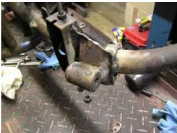
butted against the bottom engine mounting bracket so this made alignment easy and plenty of contact for welding. I was concerned about the small contact area at the front so added a metal loop having first checked it would not foul the engine. Surplus metal was then cut off with the angle grinder. The final result can be seen below.
