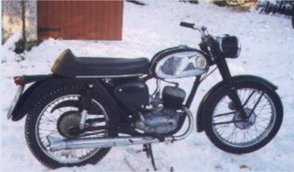
This is the 1966 D10 model with 3 speed gearbox. When acquired it had a 150 D3 motor, Fortunately, I did have a spare D10 motor to make it more original. Head is the central plug type as fitted to B175s. Makes a surprising difference to power output.
