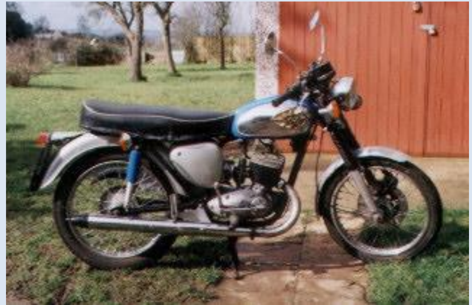
This is my Bantam special. It's built out of all the good bits I had left over after 18 months of intensive Bantam rearing. I decided to indulge my fantasy on what BSA should have done to update the Bantam. Most of the bits are BSA, the forks and disc front brake are from a Z200 Kawasaki. Barrel has been ported and it has a George Todd head. Goes, handles and stops well. One of my favourites for short journeys.
