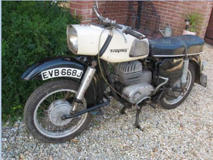
Hi level pipe and silencer are standard TS250 items cut/welded (by a friend). Tank is from an ETZ125. Headlight from an old British bike (possibly a late 250 BSA). Engine is a standard TS250 5 speeder with a 4 speed head. Tested only round the garden so far but with a 15t sprocket it seems to pull very well.
